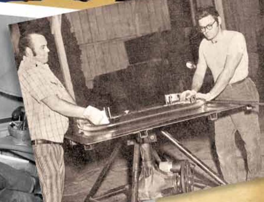
Employees Bill Usry and Dave Garner wind a coil for a custom made air conditioner at Technical Systems Incorporated in 1972.
